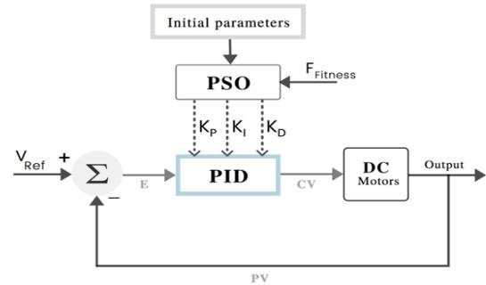
Fig. 5. Block diagram of our PID controller with PSO algorithm. Adapted from Hashim & Mustafa (2020).
