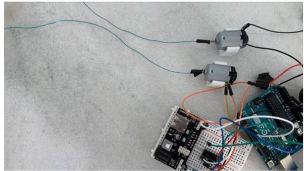
Fig. 7. Close-up shot of the *Liminal Tones* control system using an Arduino board.
