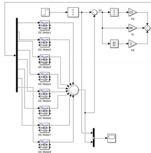
Fig. 6. Simulink block diagram of our PID controller and 8 DC motors.
